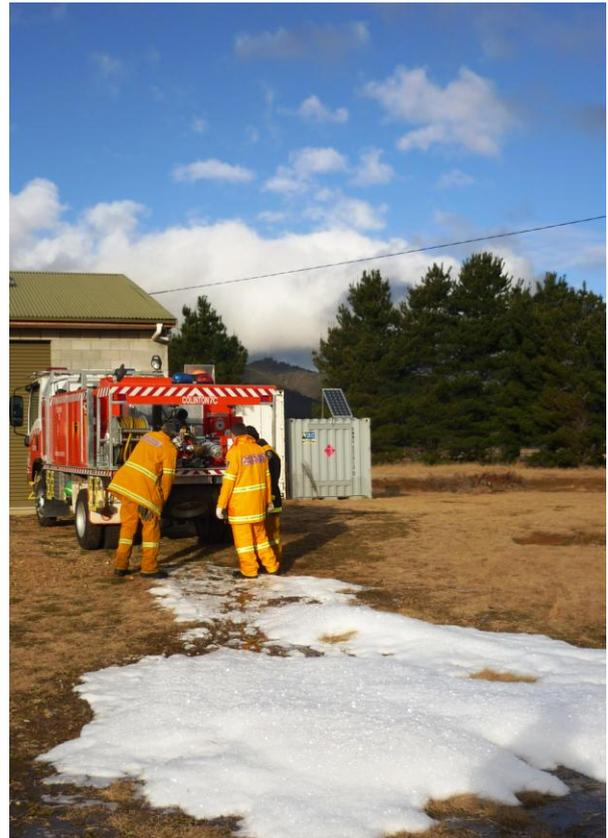
*Training: foam in the water tank prevents the pump from working. The foam (which is environmentally benign) has to be flushed out*
